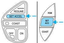
• Accelerate with your accelerator pedal. When the desired vehicle speed is reached, press and release SET/SET ACC/SET ACCEL.
